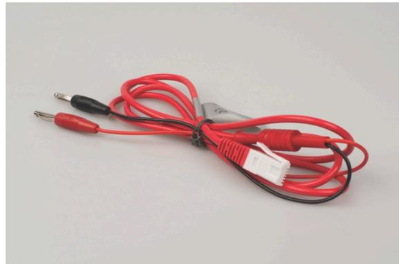
To measure a potential difference between two points in a circuit, connect the red and black plugs to the two points. A positive reading means the red plug is at a higher potential than the black plug.
