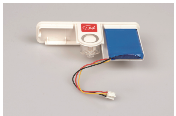
Backside of CLAB with a battery placed in its battery compartment.
