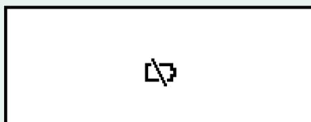
If this screen appears, replace the battery as soon as possible. For details about battery replacement, see ["Replacing the Battery" \(page 141\)](#).
